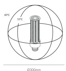
Approximately spherical, thin (1-5mm) glass or plastic diffusers Max external temperature: 40°C outside diffuser
