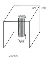
Approximately cubic, thin (1-5mm) glass or plastic diffusers Max external temperature: 40°C outside diffuser
