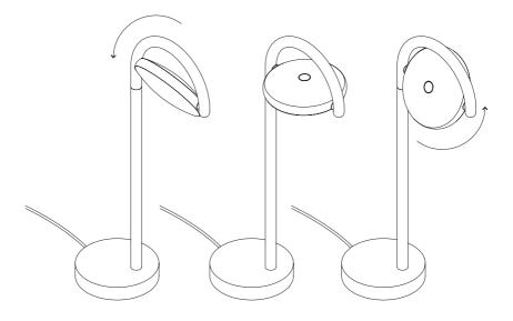
The lamp's head can also be rotated almost 360 degrees around its upright.
