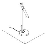
aim the fixture, 360° rotation, 90° inclination
