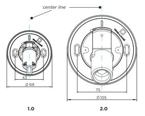
When installing, please make the center line perpendicular to the ground.
