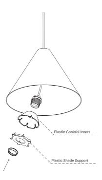
Place the shade over the bulb holder, ensuring it is parallel to the floor.
