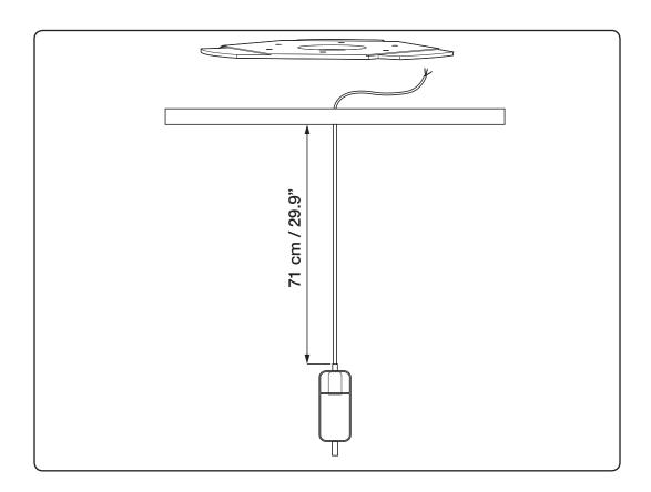
Pull the cord through the hole in the ceiling plate. The cord should measure about 71 cm / 29.9"- measured from the plate to the socket.
