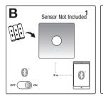
Purchase the Nordlux Sensor. Put the battery into Sensor. Turn on the Bluetooth of your phone. Stay within 8 meters from the Sensor
