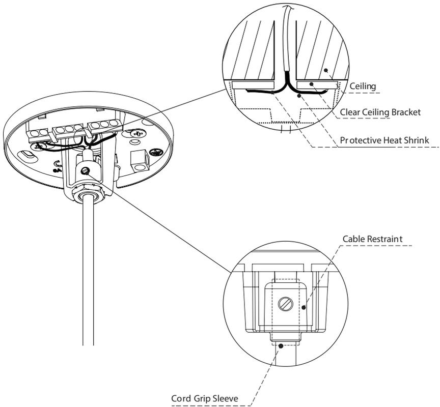
If utilising the mouse hole cable exit, please note the internal cable restraint and integrated cable clamp. The cable clamp tab can be removed and cut to the desired length to suit length to suit the cable thickness used, if this is longer than what is already provided.
