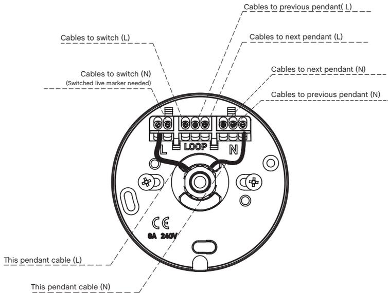
Check to ensure that the protective heat shrink, the cable restraints and cord grip sleeve are still in place after fitting all wires. Check that all of the Live, Neutral and Ground connections are securely connected before switching the power back on at the mains. Ensure there are no loose cables or exposed bare wires and that the clear ceiling bracket is securely fixed to the ceiling.
