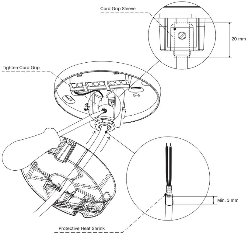
It is advised that any wire exposed with just a single basic layer of insulation is covered with the protective heat shrink provided. (Two sleeves for the basic insulated wire and one sleeve for covering the opening of the source cable).
