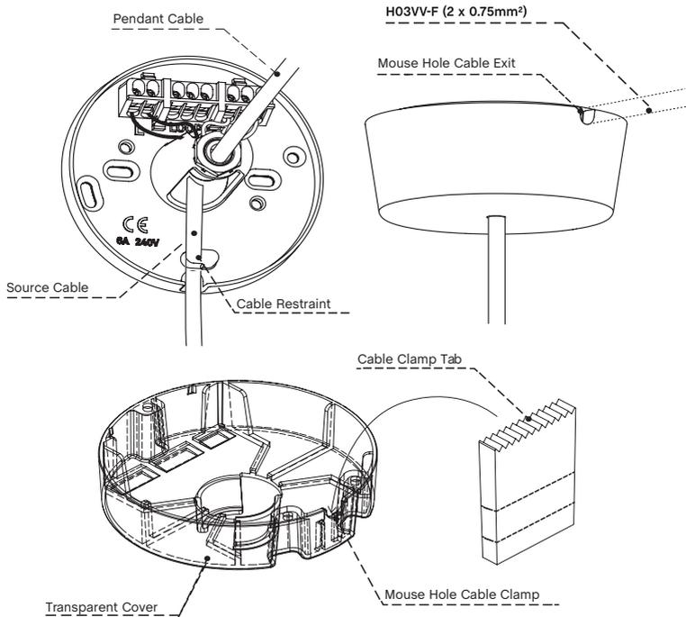
Replace the protective transparent plastic cover over the terminal and clear ceiling bracket, screwing it in place with the three fixings provided. This will isolate the internal electrics during use. Replace the outer magnetic ceiling cap over the assembly, ensuring the mouse hole exits are lined up with the cover and bracket if you intend to utilise this feature.
