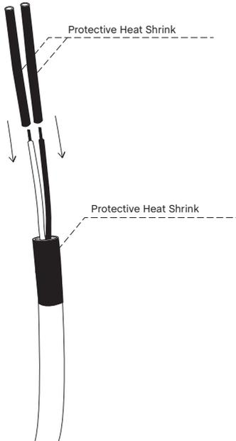
A heat gun can be used to shrink and fix this protective insulation in place, as shown below.
