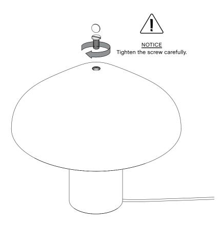
The top of the screw should be flush with the top of the shade when assembled, resulting in a visually clean side view, as pictured below.
