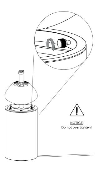
Loosen the top screw with a flat screwdriver or a small coin.
