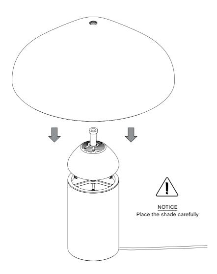
Carefully retighten the top screw with a coin or flat head screwdriver. The screw must be tightened properly to secure and level the shade. Take care not to overtighten the screw as this may damage the shade.
