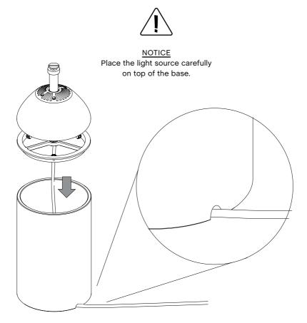
Centre the light source on the base and tighten the three screws carefully again. Tighten the screws evenly so that the light source stays centred on the base.
