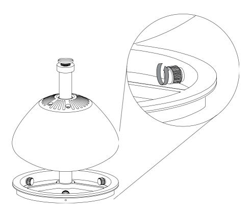
Place the light source carefully on top of the base. Pull the cable through the base, so it exits the mousehole at the bottom of the base.
