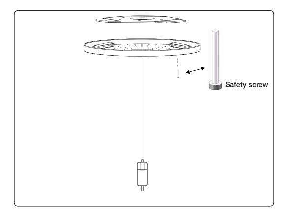
Remember to secure ceiling plate with safety screw to prevent detachment from ceiling plate.
