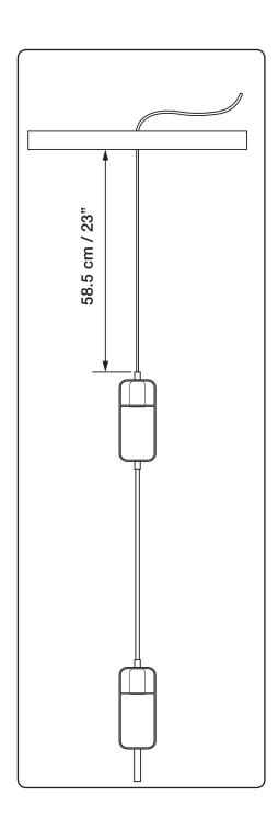
Hang canopy on to ceiling plate, securely installed into ceiling.
