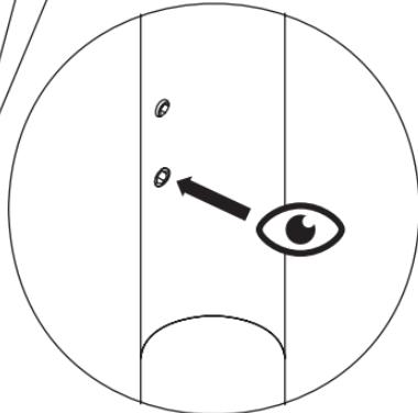
If screw is flushed with the surface, the arm can rotate freely.
