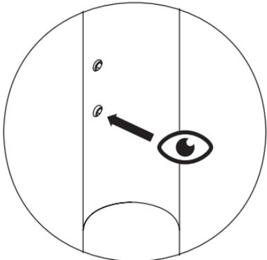
If screw is screwed into the tube, the arm is locked in the chosen direction.
