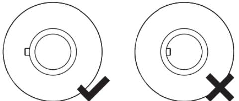
Unscrew screw until it is not visible inside (if needed)
