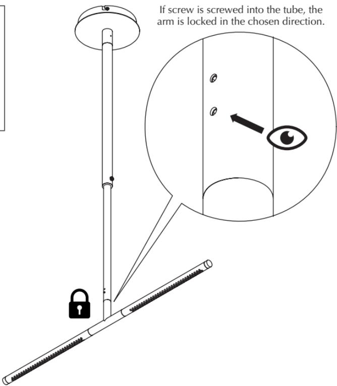
If screw is screwed into the tube, the arm is locked in the chosen direction.
