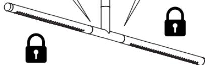
If screws are screwed into the tubes, the arms are locked in the chosen direction.
