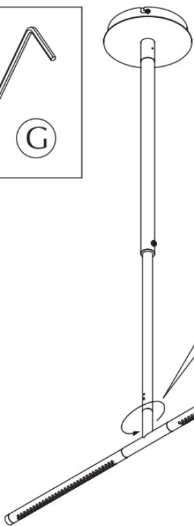
If screw is flushed with the surface, the arm can rotate freely.
