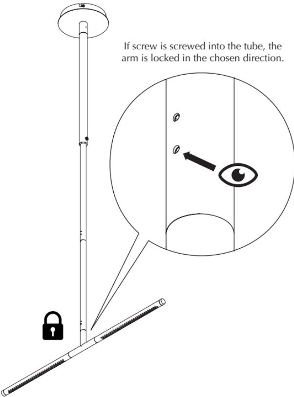
If screw is screwed into the tube, the arm is locked in the chosen direction.
