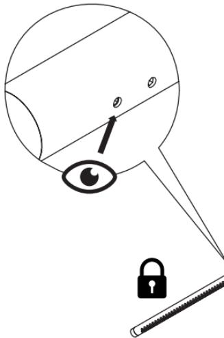
If screws are screwed into the tubes, the arms are locked in the chosen direction.
